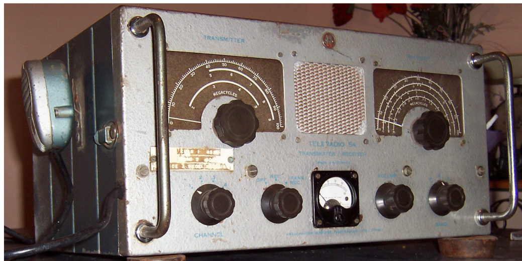
Figure 3. The front panel of the Model 5 set. The case dimensions are 19 \frac{11}{16} " wide, 9 \frac{3}{4} " high and 15 \frac{3}{4} " deep.
