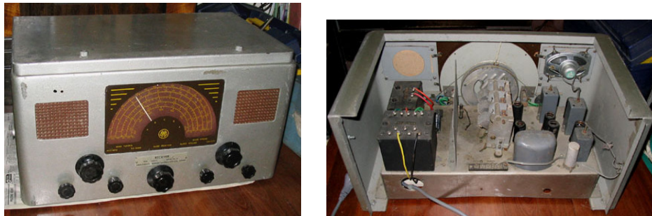
Figure 1. The Teleradio receiver Type C55163 - external and internal views [19]
