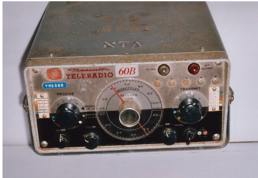
Figure 7. The type 60 A and 60B sets had the same panel layout the only difference between the two models being the transmitter output power.
