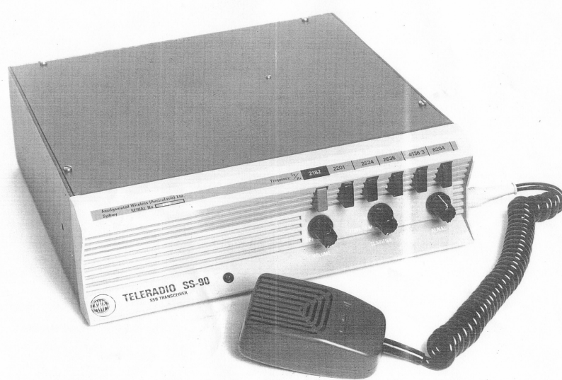
Figure 9. Rebadged Racal 7928 set sold as the SS90 Teleradio
