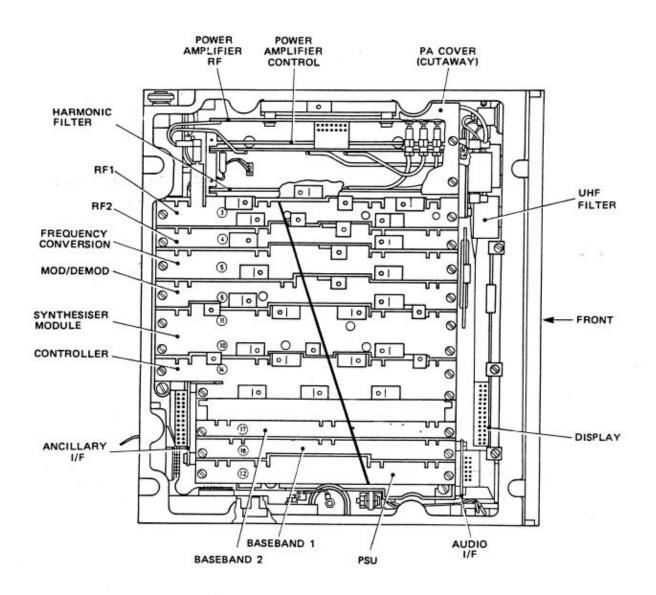
FIGURE 1 Internal View of VHF T/R
